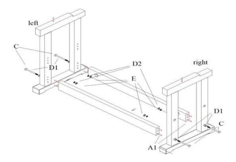
Place (insert) the cupboard on the lower stretchers of bench frame and attach the cupboard by screws - 4x40mm screws. Hint: don't glue dowels of the stretchers of bench frame. Dowel has only guide function.
